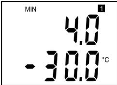
Range and type of value for output 1 (current loop II = symbol „1“ on display). Type of value, assigned to output 1, is indicated by displayed unit (here °C = temperature). Upper line displays current value corresponding to measured value (lower line). Here 4 mA corresponds to -30 °C
